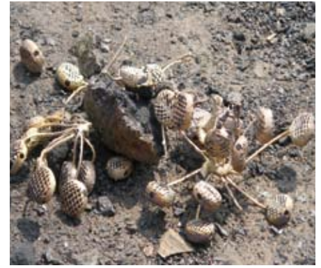
.....leaving the metal beads on the feed sprue
