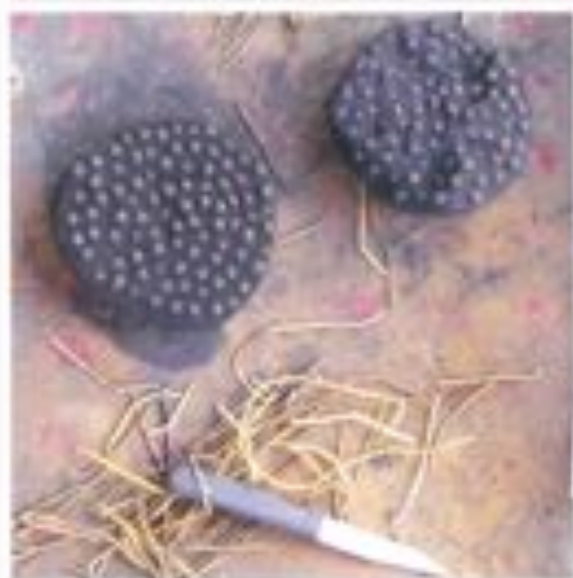
Fig 4 Wax designs pecked in charcoal with the exposed ends showing. On the table are loose wax threads.
