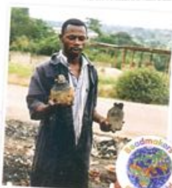
Fig 10 Break the mould and remove the beads and waste brass
