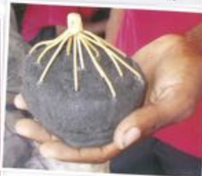
Fig 5 Wax spruce added to the exposed ends of designs in a mould, the free ends pulled together into one
